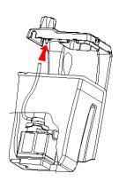
5. Connect another end of air intake hose to the silencer. Please notice to the hose should keep straight for air into smoothly.
