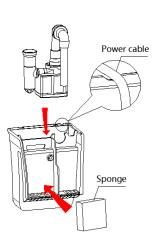
3. Put completed pump into the skimmer body, put sponge on the outlet position of body.
