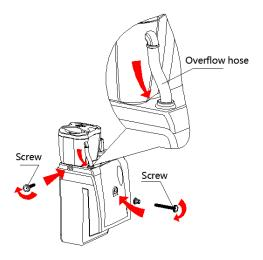
8. Fitting cover and screw on the collection cup (Notice: do not screw too over avoid to broken body).
