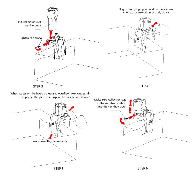
The skimmer start-up and then stop pump work, there are some water on the body and pipes. The skimmer will be work immediately when you restart to pump and needn't operate as used first time. But if body and pipe are empty as without water, we still have to operate as used first time.
