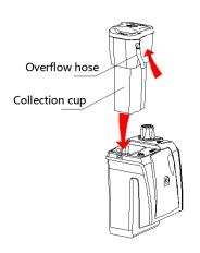
7. Collection cup put on the skimmer body and connect overflow hose to the elbow on the cup.
