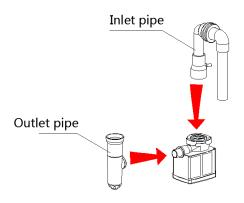
1. Insert outlet pipe into pump' s outlet and inlet pipe insert to pump' s inlet.
