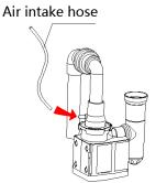
2. Connect air intake hose with air intake fitting on the inlet pipe.
